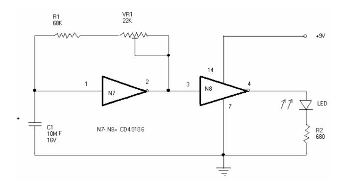
This simple circuit , 'seconds flasher or blinking activity indicator ,as it is commonly known, can be used with clocks. This circuit is built around the IC CD40106 , popularly used in clock modules.
